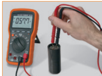
Measure Large Capacitors
