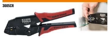
Crimps insulated terminals onto 10-22 AWG, 0.5 - 6mm2 stranded copper wire. Suitable for red, blue and yellow terminals. Unique cavity design provides consistent crimp from either side of the tool. Dial adjusts the amount of force applied to the crimp. Dual-material moulded grips provide added comfort.
